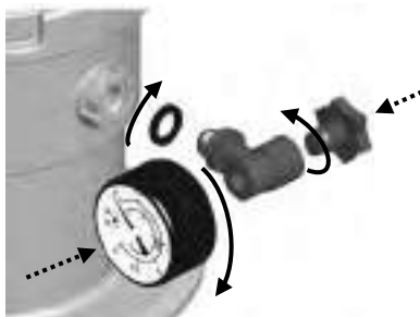
Assembly of the manometer (with valve)
